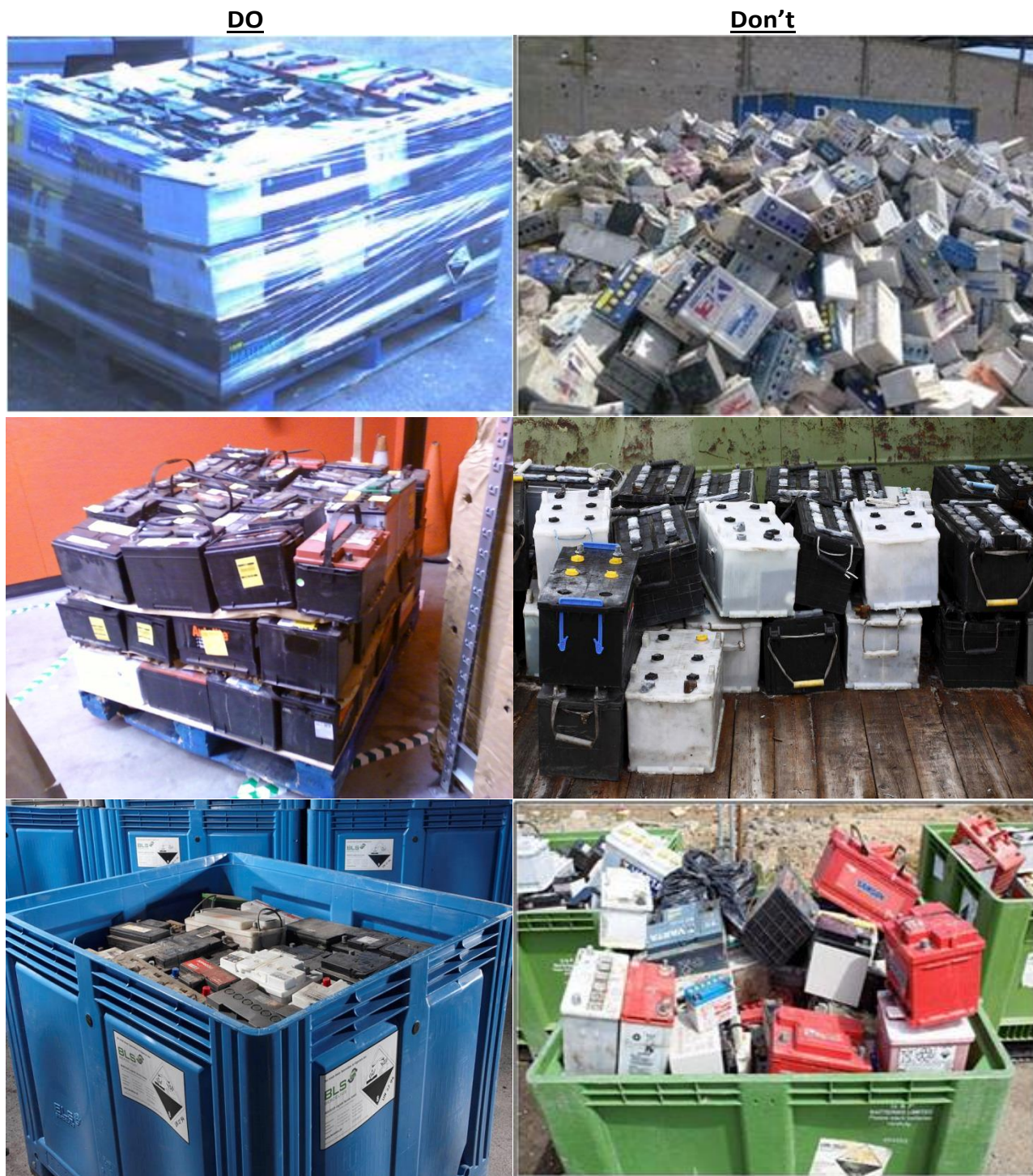
Figure 3-3 good practices Vs bad practices for temporary on site storage of UB
